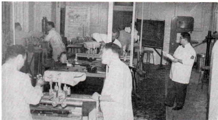
Following his demonstration of duplicating a limb on the alignment duplication jig, Instructor Ed. Hitchcock guides the class through the procedure with help of Instructor George Scoville.
