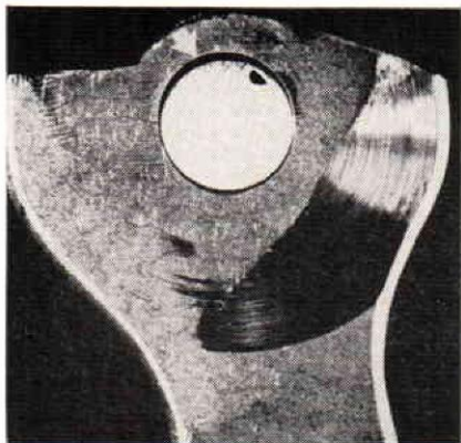
Fig. 5. Wear on Surface and in Bore of Brace Joint.
