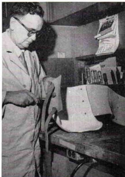
Figure 6. Fitting Technique Outline for Hemi-Pelvectomy Socket.
