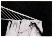
Bar A-B-C is \(^3\)\section-inch x 1/16-inch steel, heated and bent to desired angle at B. Uprights are 1/16-inch drill rod, soldered on to base B-C at 90-degree angle \(^3\)\scrip-inch apart, also soldered onto top bar A-B, all uprights being parallel. The last upright at A-C is bent up so ruler D moves under it.
