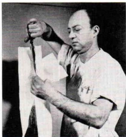
Fred Cipolla, VAPC technician, measures and trims a length of Dacron Fiber blanket, to the dimensions of standard b/k leg mold. The blanket is then stitched to form a "sleeve."
