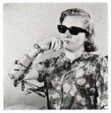
Figure 14—System providing elbow flexion and shoulder abduction for patient.
