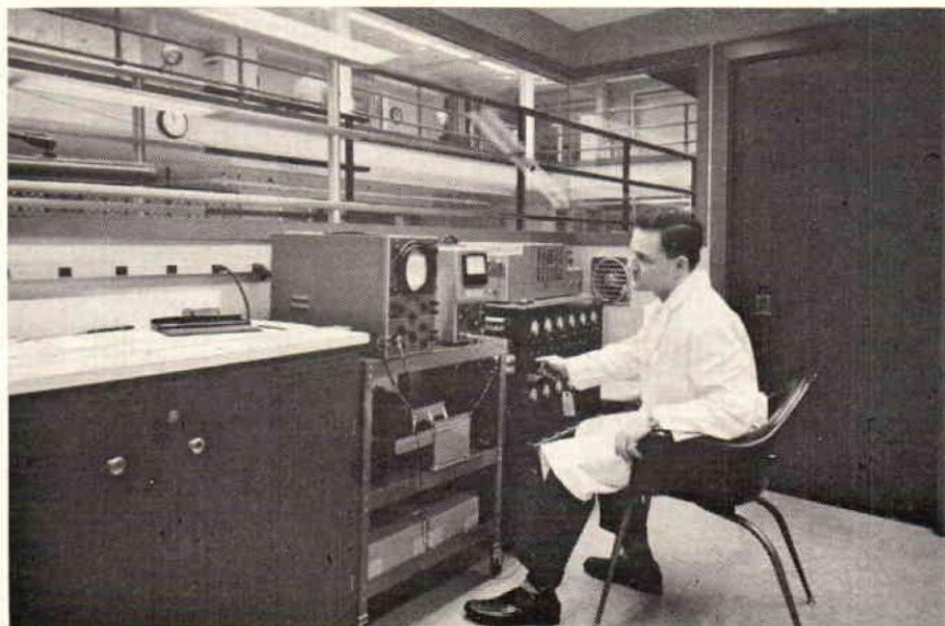
Figure 4. Instrumentation Room: Nerve center of the laboratory where all electrical outputs are monitored and recorded and where multiple data collecting devices are synchronized.
