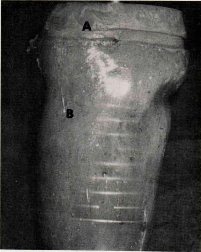
FIGURE 17. —Agar-agar stump model—A—inside of poly methyl methacrylate check socket—B.
