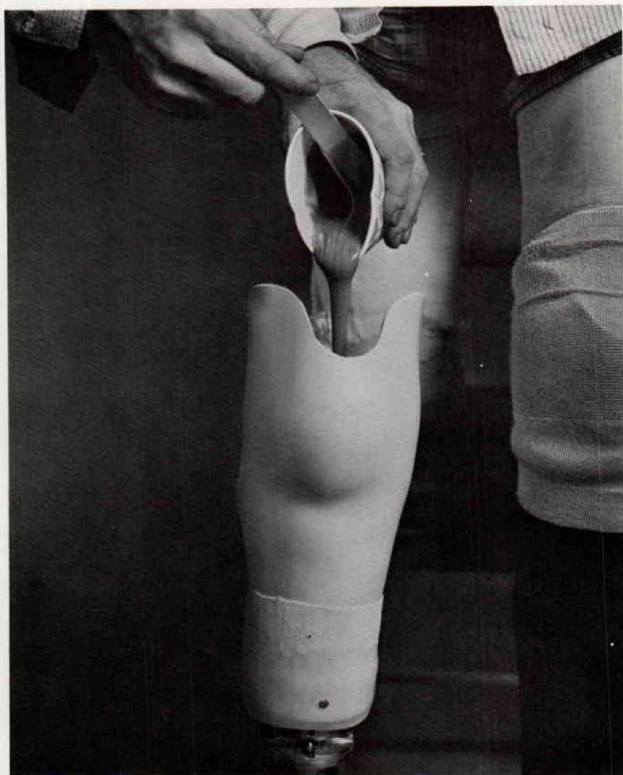
FIGURE 20—Pouring Foam Mixture to Form Total Contact Socket Bottom.
