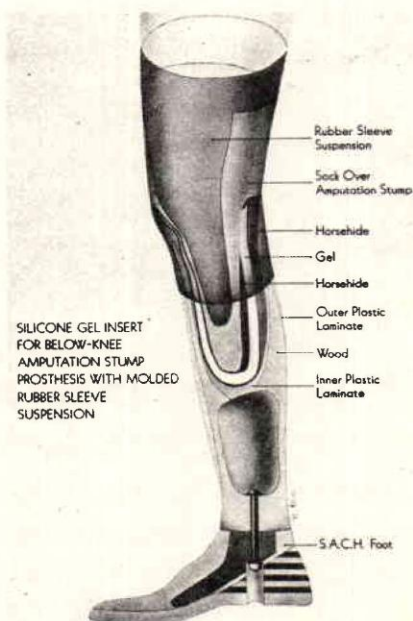
FIGURE 1—Silicone gel insert for below-knee amputation stump prosthesis with molded rubber sleeve suspension.
