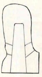
Drill air passages in the undercut areas from the outside surface to the cavity formed by the mandrel. A steel wire approximately 1/16-in. in diameter makes a good drill.
