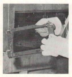
Place a 12 in. x 12 in. sheet of polycarbonate in the metal frames. Material  $\frac{3}{8}$ -in. thick is satisfactory for most adults. Material  $\frac{1}{4}$ -in. thick should be used for children and lightweight adults.
