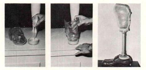
Socket is bonded to a Lexan disc approximately one inch thick—four inches in diameter. Using a burr on the router, a cavity is made to accept the end of the socket. A three-part cement <sup>5</sup> is mixed and poured into the cavity of the mounting block. The socket is held in slight flexion and adduction until the cement sets. The mounting block is then drilled and tapped and the pylon is screwed to it.
