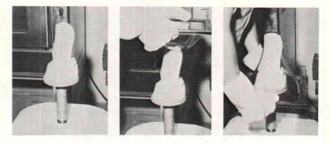
Place the heated male model on the stand. Drape the material still in the frame over the male model, push downward until the polycarbonate contacts the plywood base supporting the male model, and apply 27'' Hg vacuum. (Even better results seem to be obtained when the frame and material are turned  $180^{\circ}$  about the horizontal axis, eliminating the invagination process. It is felt that there is less tendency for formation of built-in stresses when this procedure is used.)
