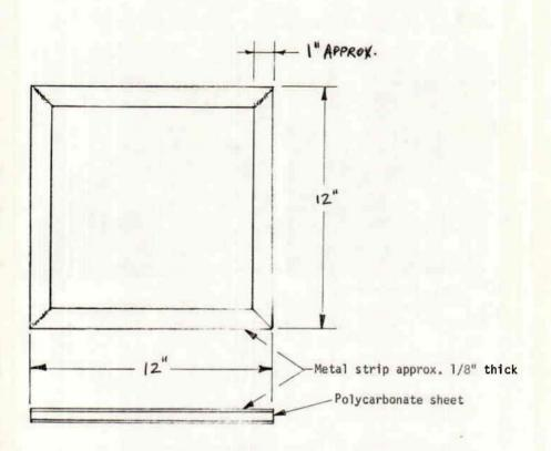
To permit proper handling of the polycarbonate sheet when heated, it is necessary to hold it in simple metal frames. Strip metal about 1/8-in. thick and inexpensive "C" clamps were used in the development program.
