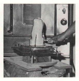
If webs form at the base, use pliers to pinch the sides together so that the inner surface is smooth.
