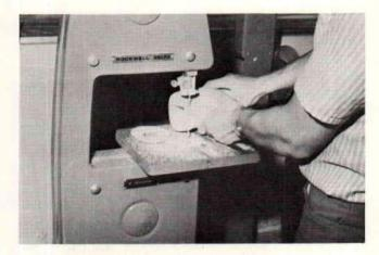
Remove the mandrel, provide a flat surface over the proximal end by sawing or filing to provide a good base for the male model during the molding phase.
