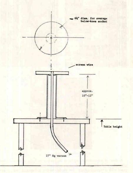
No special equipment is required other than a workstand that will support the male model so that vacuum can be applied during the forming process.
