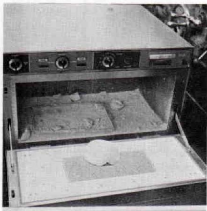
FIG. 6 Higher-powered Litton oven generated steam of water in center of cast causing same to explode as shown. Time was less than five minutes. There was no damage to personnel or equipment.
