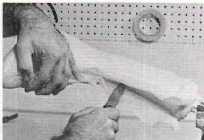
FIG. 7 Removal of the molded polypropylene from the model.
