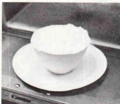
FIG. 4 After four minutes the outer surface of the plaster model was warm, damp, and water vapor was arising from the surface. There was a moderate drop in weight due to vapor loss.
