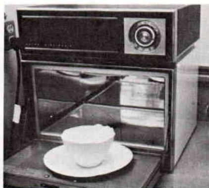
FIG. 3 Models were placed on standard paper picnic plates and energy was applied in increments of four minutes. Between each application the model was removed from the oven, weighed, replaced and drying continued.
