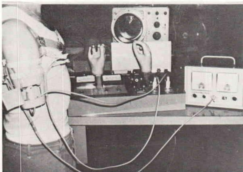
Fig. 1. The myometer used for training the patient in control of the prosthesis.
