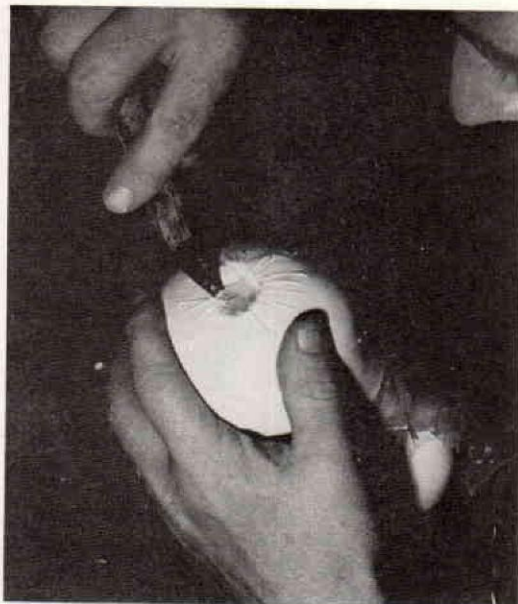
Fig. 12. A hole is cut in the socket end to provide escape for melted wax.
