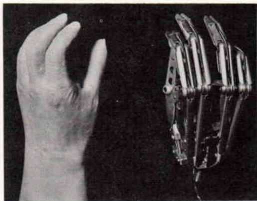
Fig. 1. EXPERIMENTAL POLYVINYL CHLORIDE GLOVE AND ARTICULATED ARTIFICIAL HAND—The NPRL molded polyvinyl cosmetic glove was individually colored at time of fabrication to match the skin tones of the patient.
