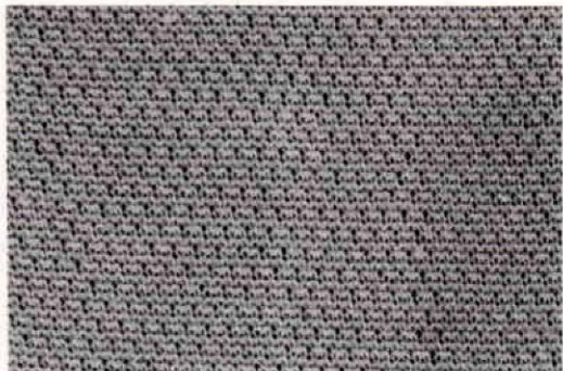
Weave structure of the Daw nylon sheath.
