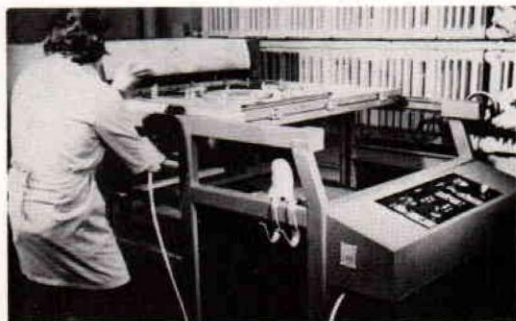
Fig. 4. The VAF machine. This model accommodates a 3-ft. sq. sheet of plastic.
