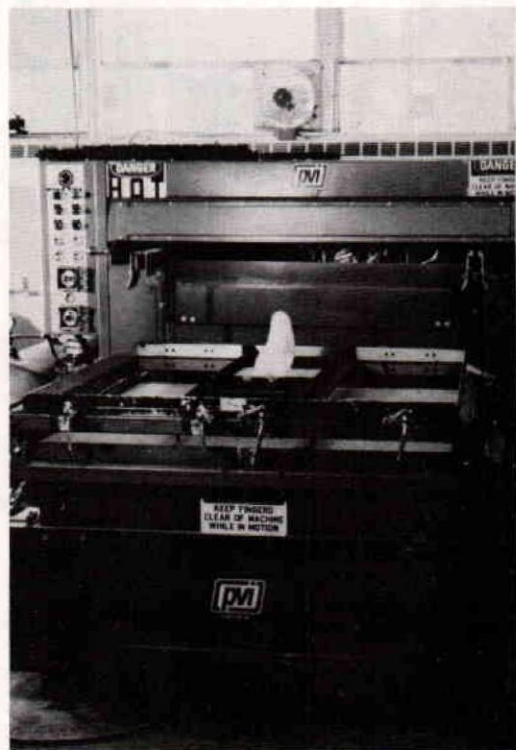
Fig. 5. The Plastic VAC machine. This model accommodates a 4-ft. sq. sheet of plastic.
