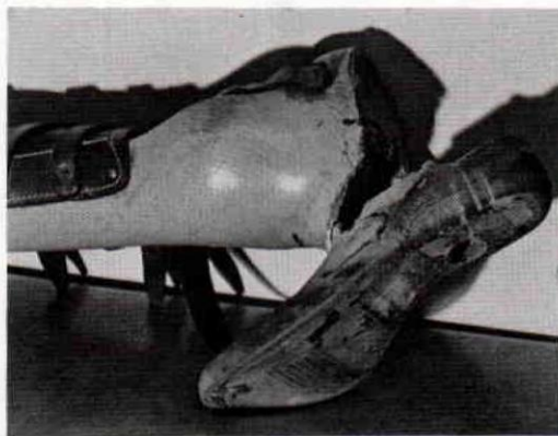
Fig. 1. Typical failure between socket and foot in posterior-opening Chopart prosthesis of standard construction.
