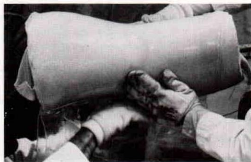
Fig. 2. One person molds the sheet over the upper surface while the other molds the sheet over the lower surface.
