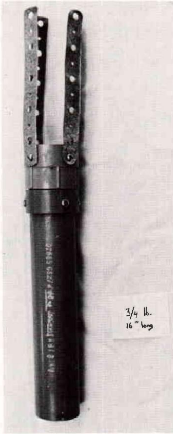
Fig. 2. An assembled pylon with galvanized straps.
