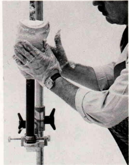
Fig. 7. Impregnating the stockinette with polyurethane resin and silica powder.
