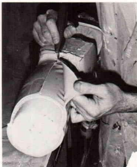
Fig. 8. The laminate is cut to the Mylar strip.
