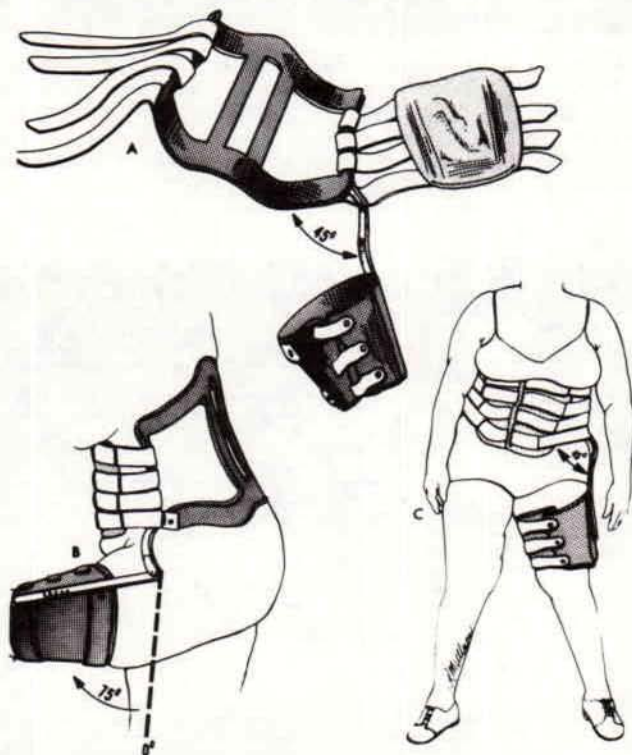
Fig. 1. Details of the orthosis. Flexion of the lower limb can control up to 75 deg. according to the case. It is advisable not to allow more than 60 deg. of flexion following a Charnley type of total hip arthroplasty.
