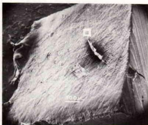
Fig. 3. Low magnification SEM of fracture surface. Area in white square presented in Figure 4.
