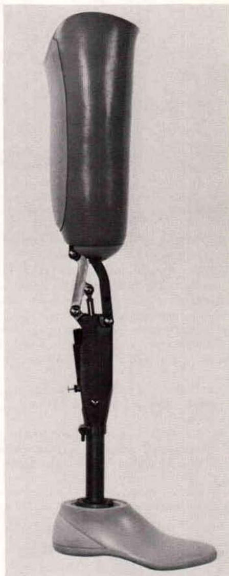
Fig. 1. The OHC knee-disarticulation prosthesis in extended position but without cosmetic cover. Note the polycentric hinge arrangement that makes it possible to place all mechanisms distal to the end of the stump and at the same time allow for installation of a fluid-type swing-phase control unit. The piston rod can be seen between the two vertical links of the four-bar polycentric system.
