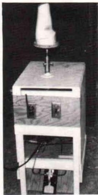
Fig. 3. Work stand with stump model on 20 cm. (8-in.) diameter support surface. Two controls are provided, the vacuum foot valve close to the floor and the electrical on-off switch for the pump near the top. Parts of the pump and ballast tank are visible at the center.
