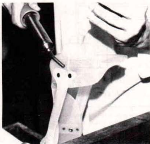
Fig. 2. The welding rod is held at 90 deg. to the seam when the round welding tip is used.
