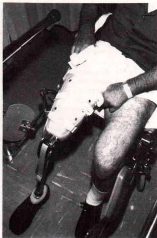
Fig. 1. Patient donning the prosthesis. Note the adjustment straps that compress the anterior and posterior socket panels.
