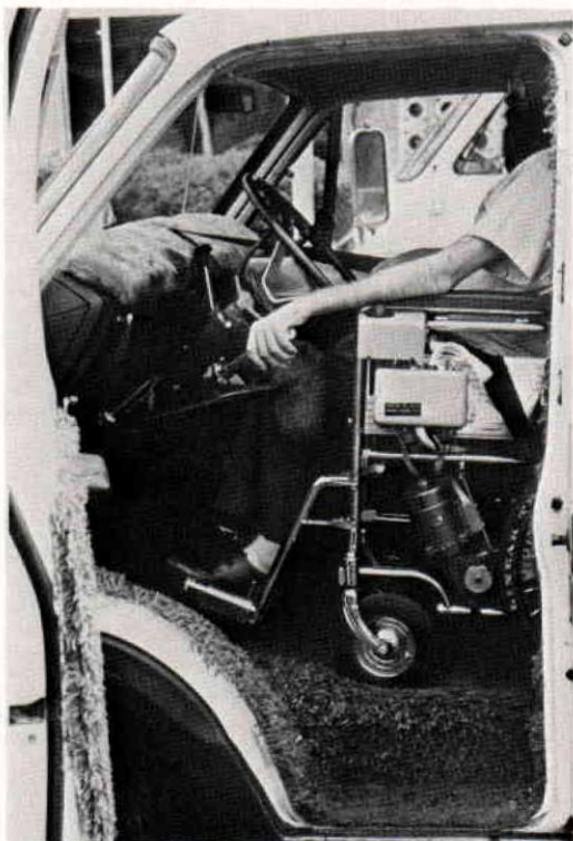
Fig. 4. A major contribution through rehabilitation engineering is the development of a multitude of vehicles that can be operated independently by severely handicapped persons.
