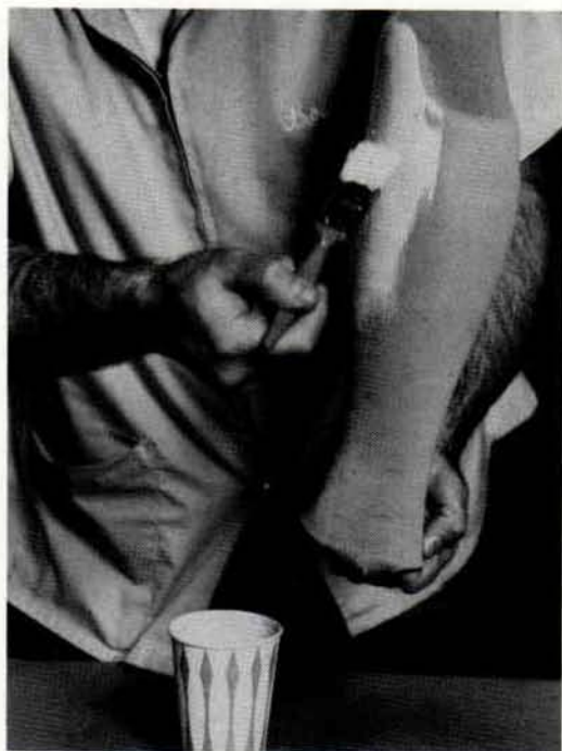
Fig. 3. One dampened cosmetic stocking is pulled over the SACH foot and foam cover (in the example, a Hydra-cadence cover is shown). The stocking is tied at the top and suspended. The acrylic latex is then painted, on, using smooth, even strokes. Each layer should be sanded lightly when drying is uneven before application of the next coat. Three or four coats are required, with a drying time of one to two hours between coats. (Courtesy of the Veterans Administration Prosthetics Center).
