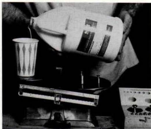
Fig. 2. Mixing the acrylic latex. The proper color is determined by matching the shade guide to the patient's skin. Instructions on the shade guide (Fig. 1) explain the proper ratios to mix. About 200-300 grams of acrylic latex are required to coat a below-knee prosthesis. (Courtesy of the Veterans Administration Prosthetic Center).
