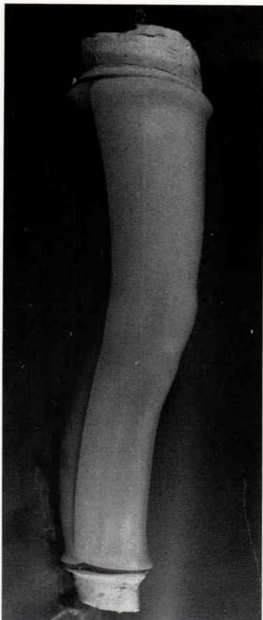
Fig. 11. Anterior section vacuum formed, trimmed, and reassembled on the model with the posterior section.
