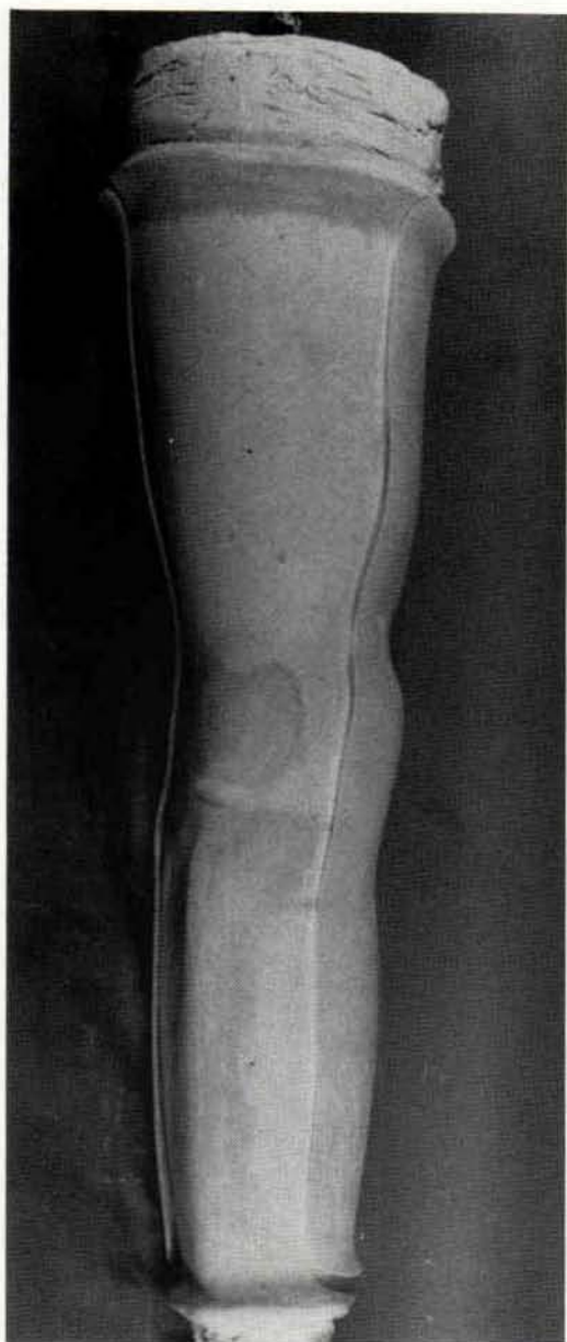
Fig. 10. Posterior section of the orthosis once it has been vacuum formed, trimmed, smoothed, and re-applied to the model for vacuum-forming of the anterior section.
