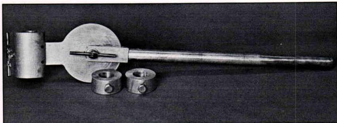
Fig. 2. Universal Positioning Arm. Two locking rings are shown in the foreground.
