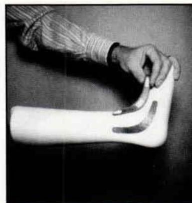
Figure 4. The insert is held in place on the mold with 1/32 inch thick Scotch mounts; three small pieces above the insert and provide some space under the insert.
