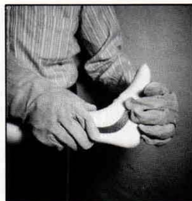
Figure 3. The carbon composite insert is heated to 300° by using an oven or a heat gun; it is then pliable and is held in place on the mold until it cools.
