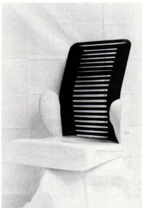
Fig. 2—Fabrication of the seat. Wide rubber bands are stretched across the back. Ethafoam and temper foam are used to pad the seat and lateral pads.
