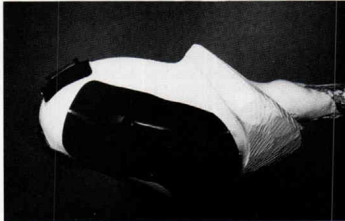
Fig. 4—The rubber/carbon electrodes were trimmed and cemented to the socket as desired.
