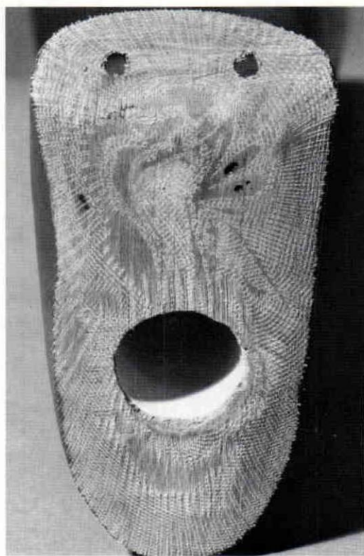
Figure 11. KEEL area sanded and \frac{1}{4} " holes drilled for bonding sole to KEEL.
