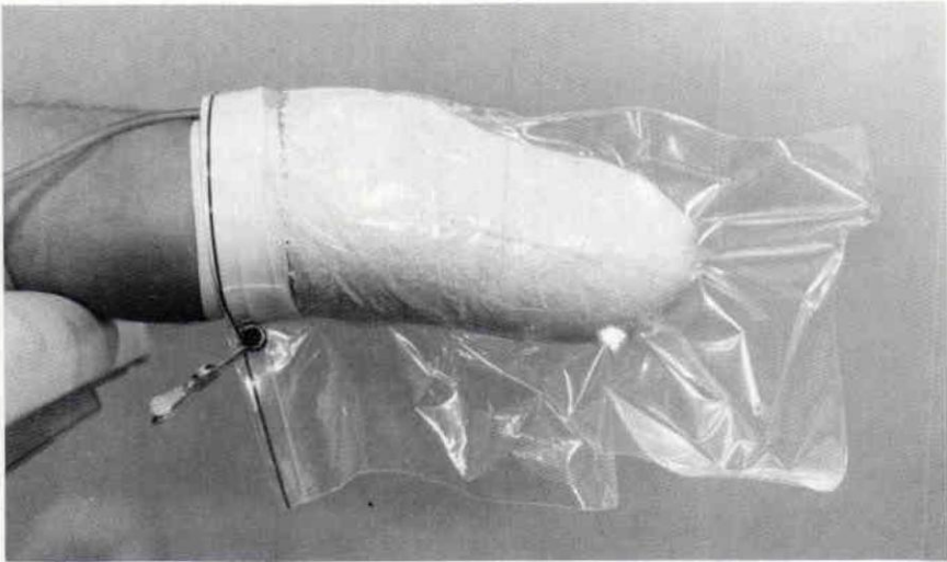
Figure 14. Apply vacuum (20 to 30 inches of mercury).
