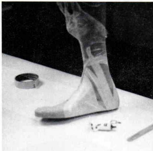
Figure 7: After the foot is bonded, the foot and ankle block are taped and allowed to cure for 24 hours.
