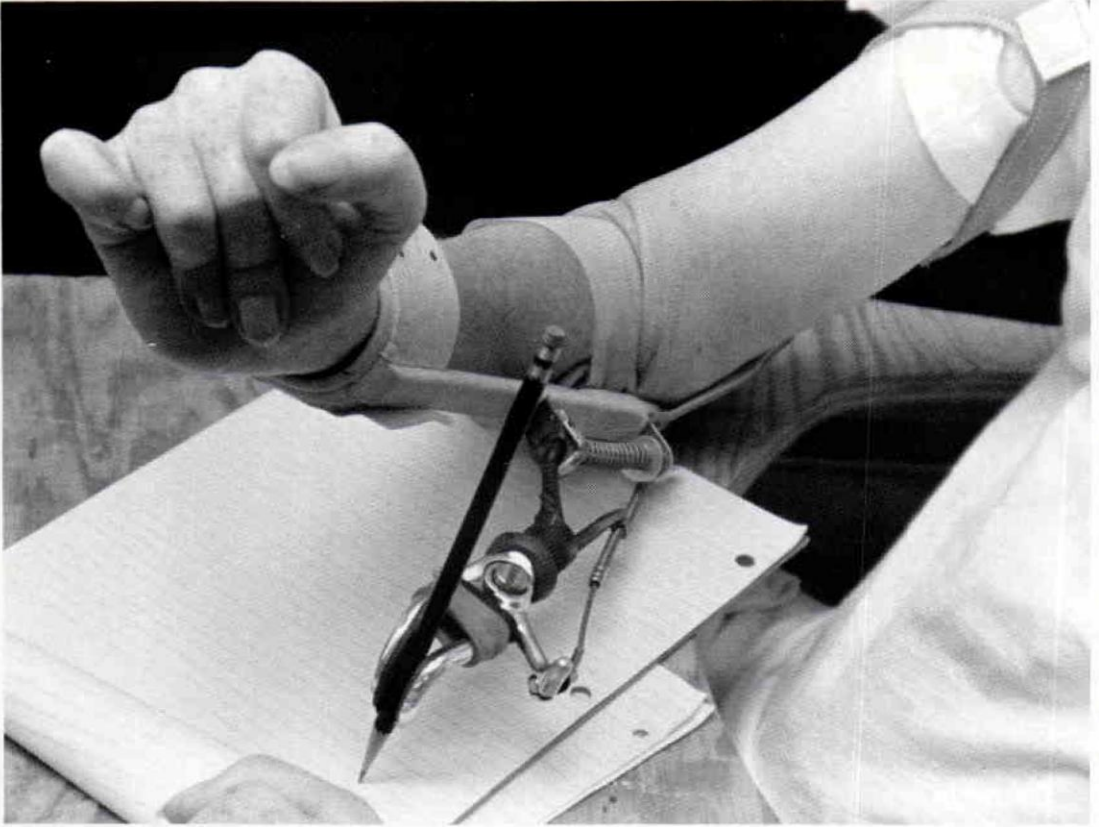
Figure 3: Closeup of hook in writing position. Bracket and rotating rod assembly can be seen.
