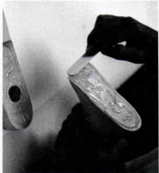
Figure 6: A smooth coat of the urethane bond is applied to the foot and ankle block.
