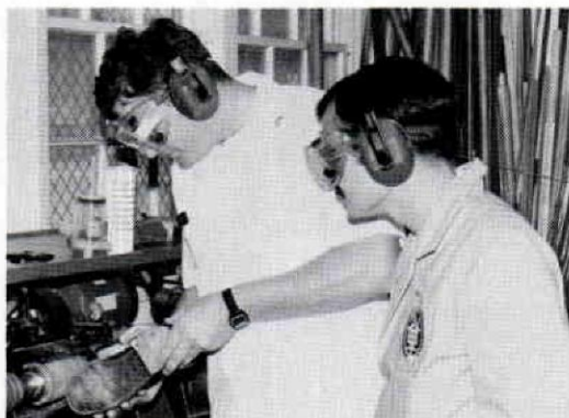
Instructor supervises a student using a shoe finisher.
