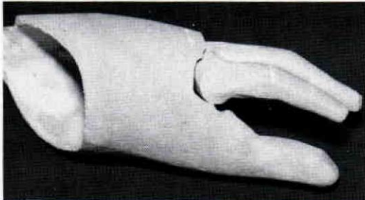
Figure 15. The rough M-P's of the finger unit are rounded smooth. The socket is then ground in a concave manner to accept the finger unit.
