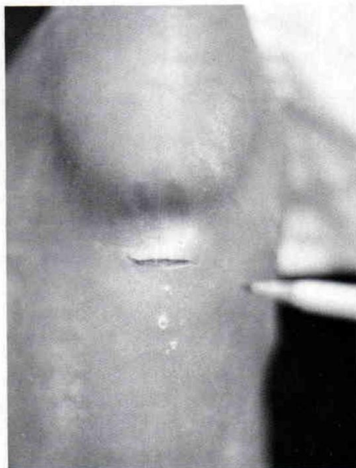
Figure 7. Common area of deterioration in hot-melt liners.
