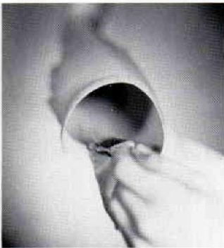
Figure 9. Bond the posterior seam together along the inside.
