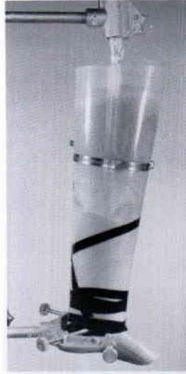
Figures 4 and 5. Fill the void with rigid polyurethane foam.
