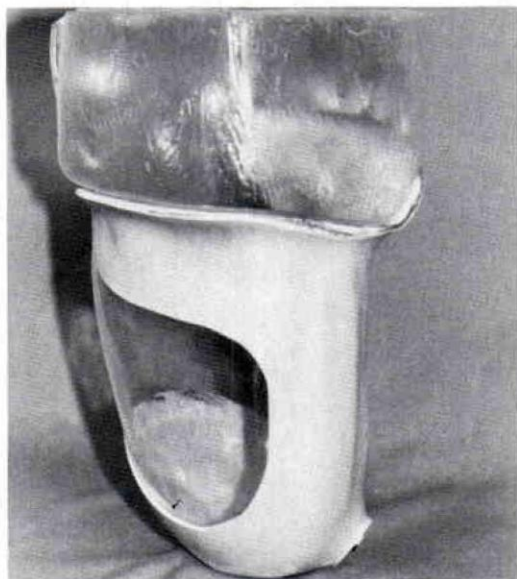
Figure 18. The laminated and rough trimmed frame in place about the Surlyn socket.
