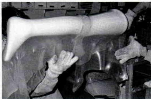
Figure 5. Continue to check for areas not sealed.
