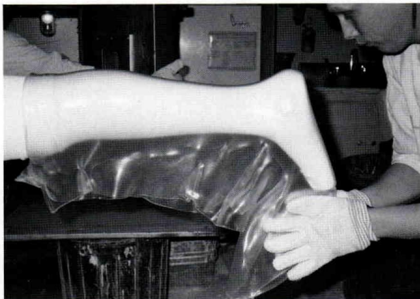
Figure 3. While one staff member seals the hot plastic, the other individual removes the proximal section from the oven.
