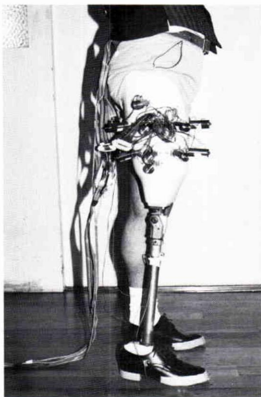
Figure 11. Lateral view, showing socket with four transducers placed along lateral wall.
