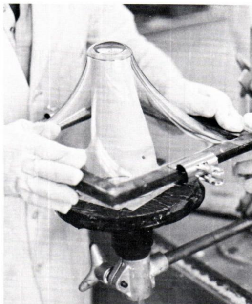
Figure 7. Molten transparent thermoplastic is vacuum-formed over the residual limb model.
