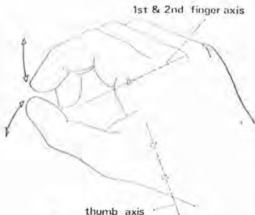
Fig. 4. Geometry of OBEU hand.
