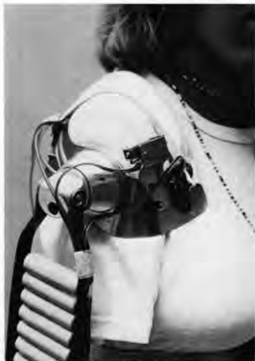
Fig. 7. Hybrid prosthesis in bilateral amelia with pneumatically lockable shoulder joint (controlled by valves in the left side) and pressure and traction microswitches for gripping and forearm rotation. Built-in accumulators fitted to the frame of the right upper arm.
