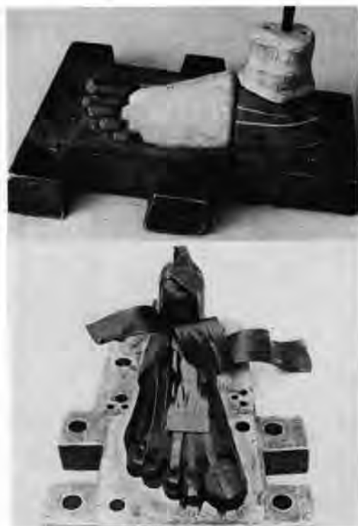
Fig. 7. Top, components of the Jaipur foot. Bottom, rayon cord, used in automobile tyres, reinforces and binds the components. Structural failures are now rare.
