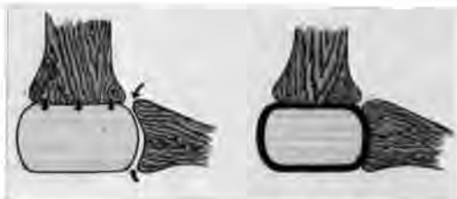
Fig. 6. Left, the proximal wooden block sinks into the unprotected sponge rubber causing damage during weight bearing. Right, enclosure in a shell of solid rubber protects the sponge rubber block; no subsequent structural failures have been encountered.
