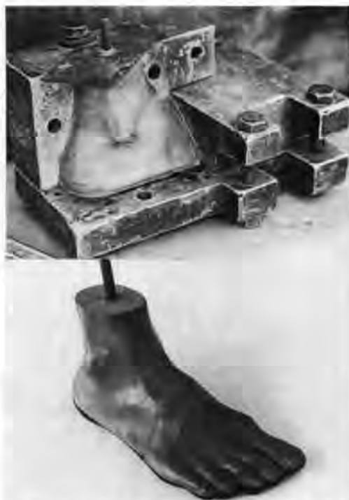
Fig. 3. Top, die prepared from plaster replica of normal foot. Bottom, cosmetically acceptable footpiece of solid rubber.
