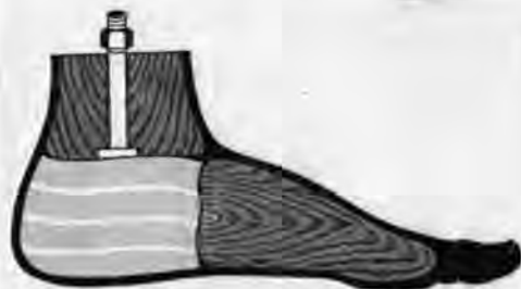
Fig. 5. Initial design of Jaipur foot.
