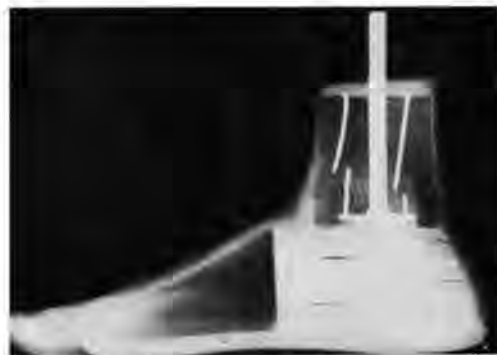
Fig. 9. The separation of the layered structure of the sponge rubber joint is shown in this skiagram, see text.
