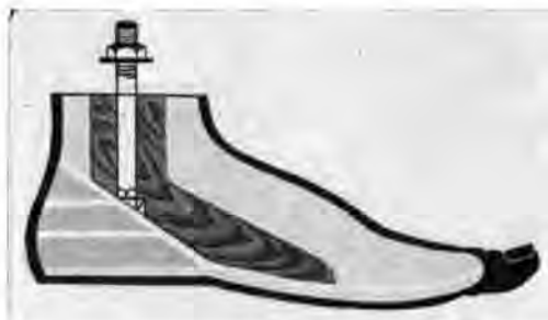
Fig. 4. Rubber enclosed SACH foot, see text.
