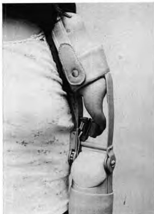
Fig. 6. Microswitch which is operated by the movements of the one finger phocomelia.
