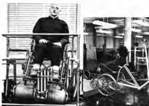
Fig. 2. Left, "One year of normal use shall be simulated by driving a chair 360 hours with a 200 lb (91 kg) anthropomorphic dummy on a series of drums that provide a surface velocity of 5 mph (8 kph) and an alternating surface angulation of 9° both drum slope to the right, inward, to the left and outward." Right, "The chair shall be driven on 6 in (15 cm) curb drop simulator with the anthropomorphic dummy for 1,800 drops one way and 1,800 in a reverse direction" to subject the wheels and frame to equal impact loading over the 3,600 drops.
