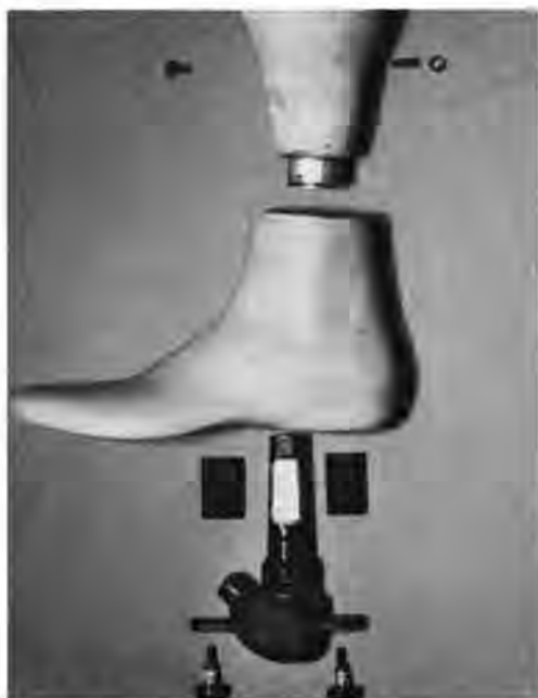
Fig. 4. The complete foot/ankle system components (bottom to top), two holding screws, hydraulic unit, two rubber bumpers, moulded foot, wood block/shin tube set-up, 2 set screws and two locking nuts.
