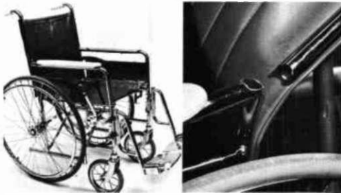
Fig. 6. Left, Lightweight wheelchair "A." Right, structural failure in "A" as a result of curb drop test.
